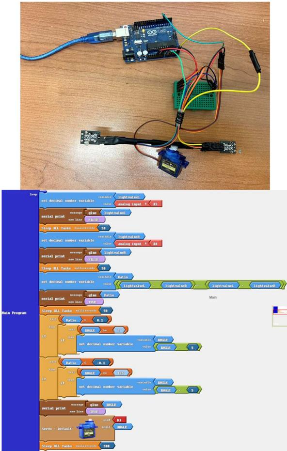
Fig. 3. A minimal chassis preparation for agrivoltaic panels utilizing two photoresistors and an angle servo (top part) and the corresponding algorithm implementation using the ArduBlock tool (bottom part)
