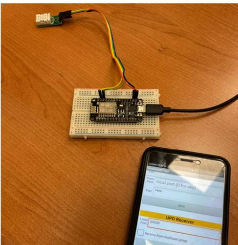
Fig. 6. Experimental IoT system for wireless monitoring of air temperature and humidity, via a smart phone
