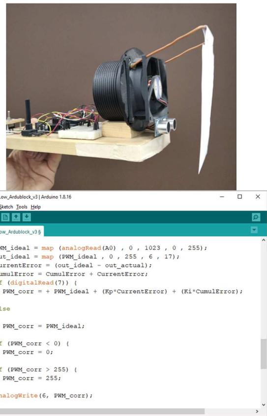
Fig. 4. Experimental controllable air flow unit utilizing the distance from a piece of paper in front of the fan as feedback parameter (top part) and an indicative implementation using the Arduino IDE (bottom part)
