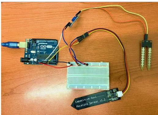
Fig. 1. Diverse soil moisture measurement arrangements utilizing cost effective sensing modules of resistive and of capacitive type
