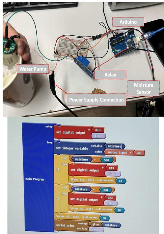
Fig. 2. On-Off control using soil a cheap soil moisture sensor module and a relay (top part) and the corresponding algorithm implementation using the ArduBlock tool (bottom part)
